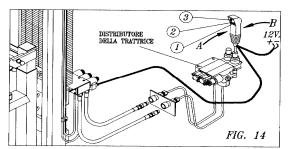
There is an alternative to the usual hand levers distributor: It is possible E.L.S. agricultural elevators work by means of a one-lever device with electric function to be mounted on the lever of the tractor double effect distributor used for elevator working.
